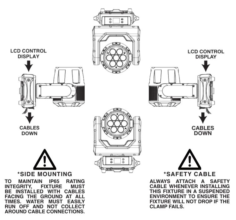
The Hydro Wash X7 is fully operational in three different mounting positions, hanging upside-down, mounted sideways on trussing, or set on a flat level surface. Always use and install a safety cable as a safety measure to prevent accidental damage and/or injury in the event the clamp fails. Never use the carrying handles for secondary attachment.
